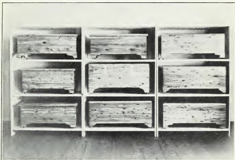
NINE CEDAR CHESTS, RANGING IN CAPACITY FROM 3.9 CUBIC FEET TO 5.5 CUBIC FEET, USED IN EXPERIMENTAL WORK.
